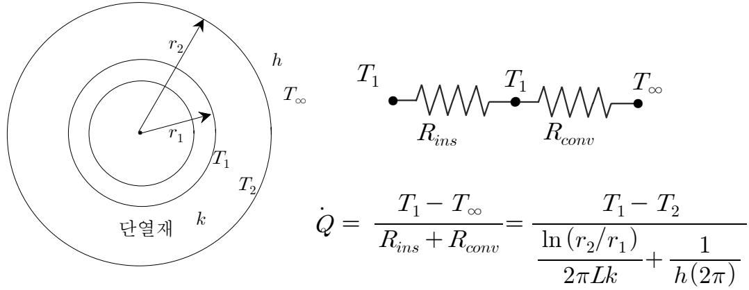
$$\begin{aligned}\frac{d\dot{Q}}{dr} &= 0 \Rightarrow r_{cr,cylinder} = \frac{k}{h} \\ r_{cr,sphere} &= \frac{2k}{h}\end{aligned}$$
