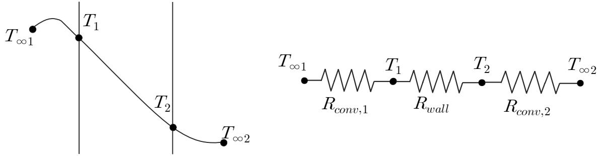
$$\dot{Q} = \frac{T_{\infty 1} - T_{\infty 2}}{R_{conv,1} + R_{wall} + R_{conv,2}} = \frac{T_{\infty 1} - T_{\infty 2}}{R_{total}}$$
