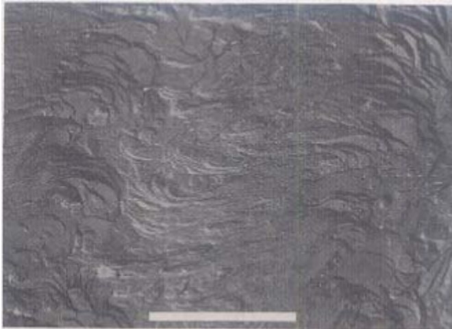
1.7 Lamellae within adjacent bands of a banded spherulite of linear polyethylene crystallized at 125°C. The specimen was cut open after crystallization, and lamellae are revealed by permanganic etching of the cut surface. The electron micrograph is of a carbon replica of the etched cut surface (after D. C. Bassett). Scale bar = 10 \mu\text{m} .
