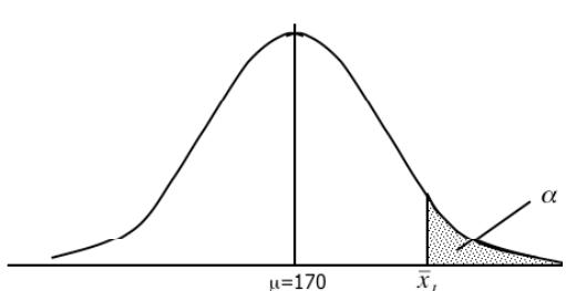
$$P\left(\frac{\bar{x} - \mu}{\sigma/\sqrt{n}} > \frac{\bar{x}_L - \mu}{\sigma/\sqrt{n}}\right) = P\left(Z > \frac{\bar{x}_L - \mu}{\sigma/\sqrt{n}}\right) = \alpha$$
